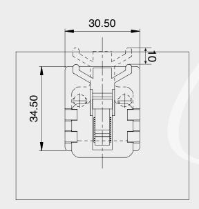
Overall dimension are in millimeters. On demand detailed drawings will be provided.
