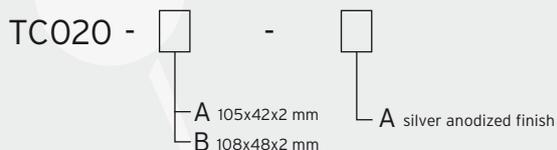
Overall dimension are in millimeters. On demand detailed drawings will be provided.
