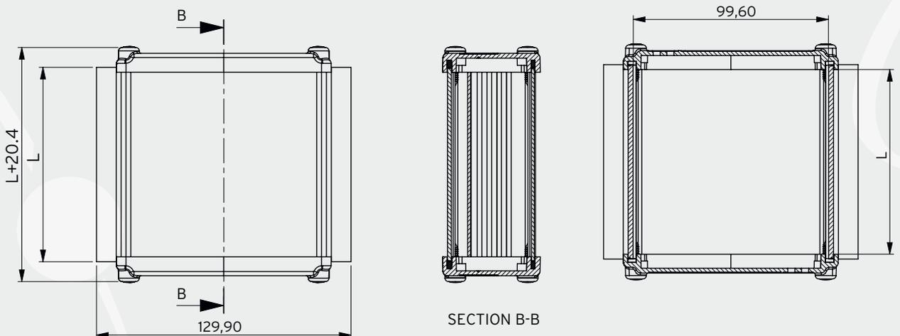
Overall dimension are in millimeters. On demand detailed drawings will be provided.
